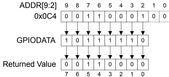
Figure 8-3. GPIODATA Read Example
