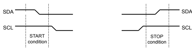
Figure 16-3. START and STOP Conditions
