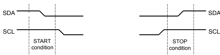
Figure 15-3. START and STOP Conditions
