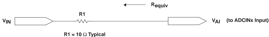
Figure 30. Typical ADC Input Pin Circuit
