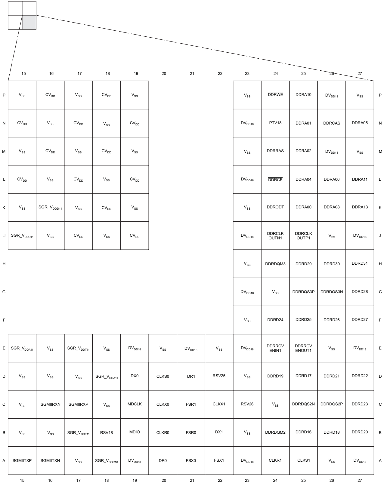
Figure 2-4. TCI6487/8 Pin Map (Bottom View) [Quadrant C]
