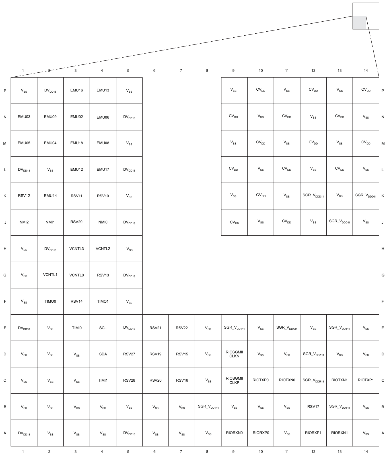
Figure 2-5. TCI6487/8 Pin Map (Bottom View) [Quadrant D]
