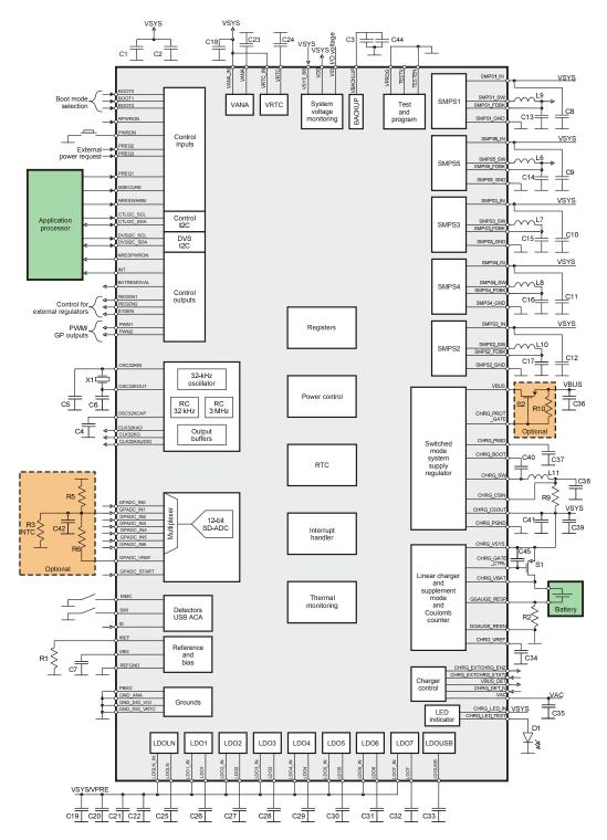
Figure 1. TWL6032 Device Block Diagram
