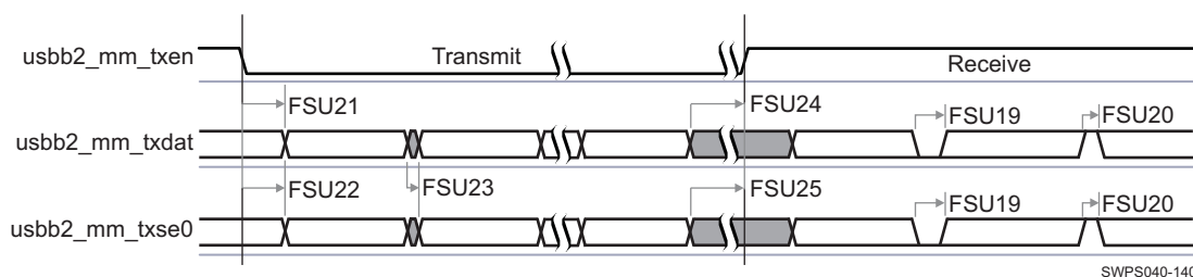
Figure 5-95. Low- / Full-Speed USB2—Bidirectional Standard 3-pin Mode—1.8 V
