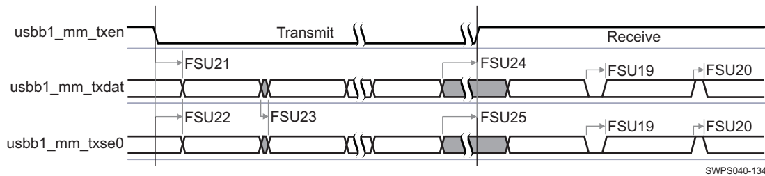
Figure 5-88. Low- / Full-Speed USBB1—Bidirectional Standard 3-pin Mode—1.8 V
