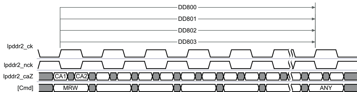
Figure 5-43. EMIF—DDR Mode—ZQ Calibration Parameters (1)(2)(3)
