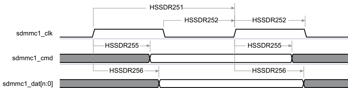
Figure 5-115. MMC/SD/SDIO 1 Interface—High-Speed SD Mode—Transmitter Mode (1)
