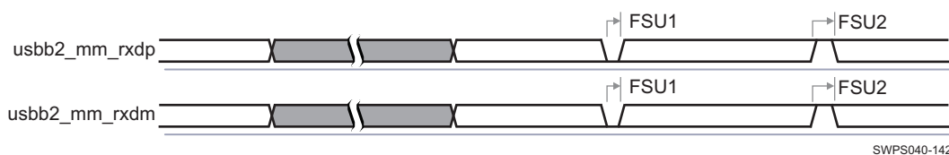
Figure 5-97. Low- / Full-Speed USB2—Bidirectional 2-pin Mode—1.8 V
