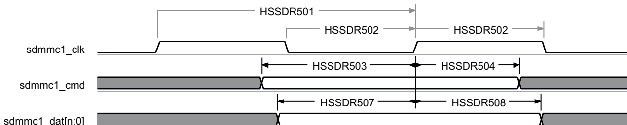
Figure 5-118. MMC/SD/SDIO 1 Interface—High-Speed SDR50—Receiver Mode (1)
