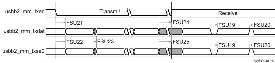
Figure 5-98. Low- / Full-Speed USB2—Bidirectional Standard 3-pin Mode—1.8 V
