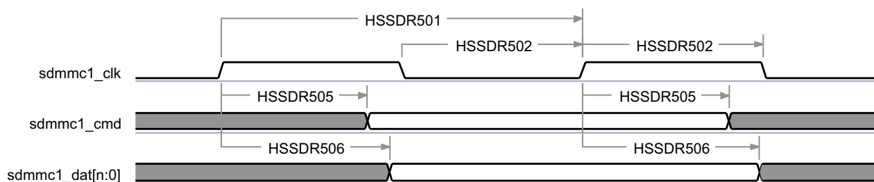
Figure 5-120. MMC/SD/SDIO 1 Interface—High-Speed SDR50—Transmitter Mode (1)
