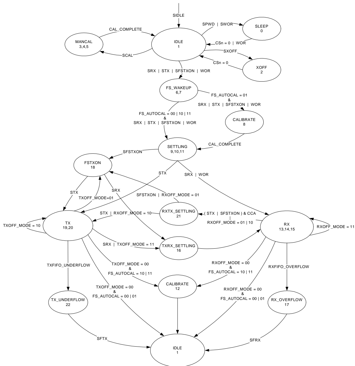
Figure 20: Complete Radio Control State Diagram
